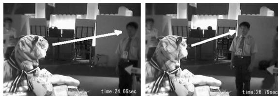
**FIGURE 12.12** The developed robot vision system named “Gazing Tiger” and its operation. It gazes at a human face by detecting the position of the face using the optical multiple-correlation system.
