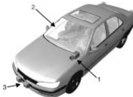
FIGURE 1.36 Optical-based smart car: (1) a video-camera-based lane-centering system; (2) a heads-up holographic windshield display for sharper night vision; (3) a sensor-based collision-warning system that alerts drivers to road hazards. (From Anderson, S. G., *Laser Focus World*, 32(6), 117–123, 1996. With permission.)
