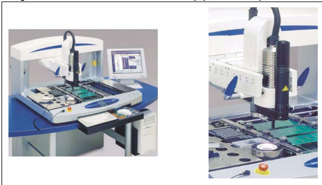
Figure 12. Comintec ONYX32 semi-automatic equipment for component rework
