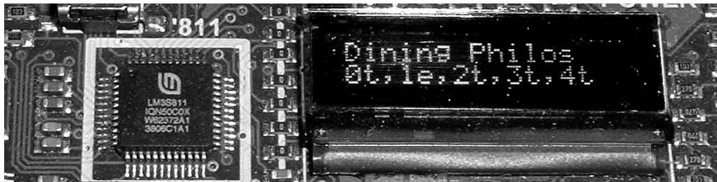
Figure 9.6: DPP test application running on the EV-LM3S811 board (Cortex-M3). The status of each Philosopher is displayed as “t” (thinking), “e” (eating), or “h” (hungry).
